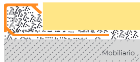
Cross-sectional image of a Schlüter®-Rondec-Step profile
